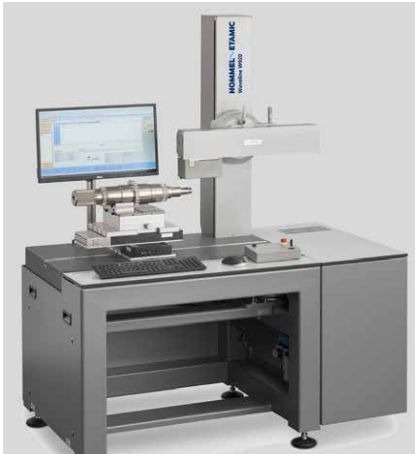
Waveline W920 with 500 mm measuring column and 200 mm traverse unit
