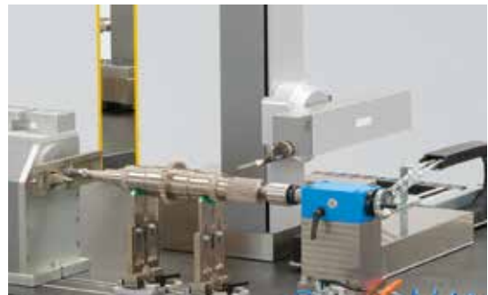
Rotating measuring column and probe rotation module for optimum access to the measuring point
