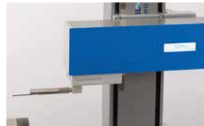
Roughness probe system with quick-change-adapter
